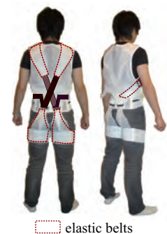
Fig.2: Passive power-assist device Smart Suite Lite.
