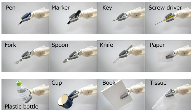
Fig. 3 Examples of daily objects grasping with the Finch
