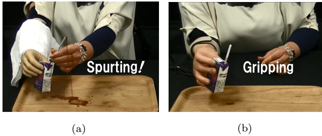
Fig. 3 Grasping of drink box. (a) Conventional artificial hand. (b) General purpose artificial hand with haptic transplant.
