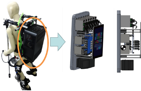
Fig.4 Control box of TTI-Knuckle1
