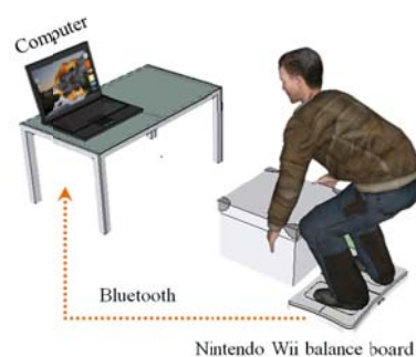
Fig. 1. An experimental overview for measuring the center of balance during lifting a load.
