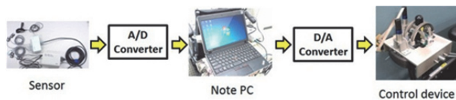
Fig.4 Configuration of the control system
