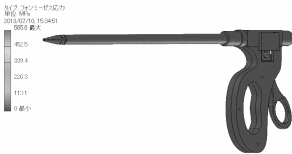
Fig. 10 Stress test result by finite element analysis
