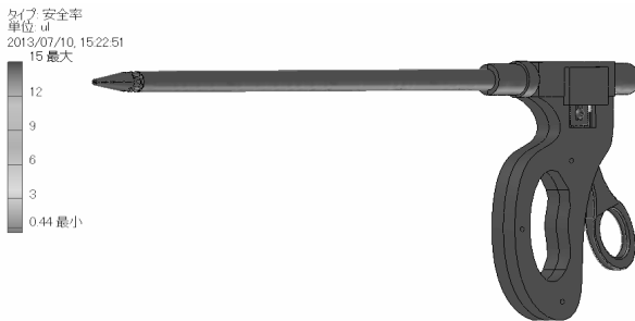
Fig. 11 Safety rate result by finite element analysis
