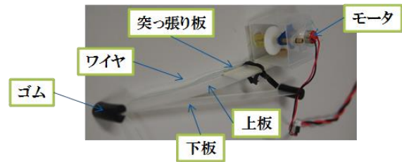
Fig. 4 Structure of balloon jump robot
