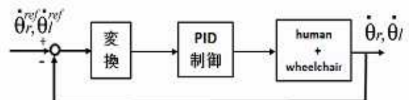
Fig. 2 Configuration of power assisting control system.
