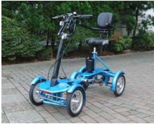
Fig. 1 Four-wheel electric power-assisted personal mobility
