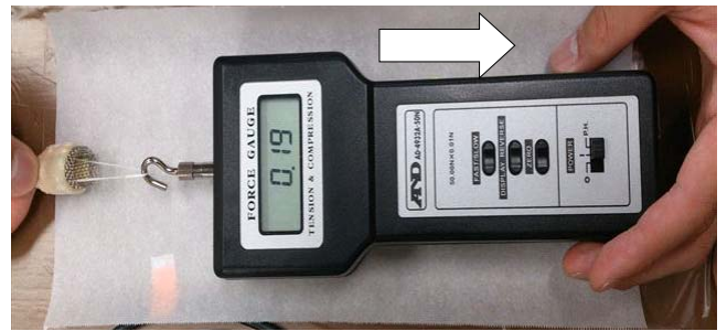
Fig. 4 Measurement adhesive strength
