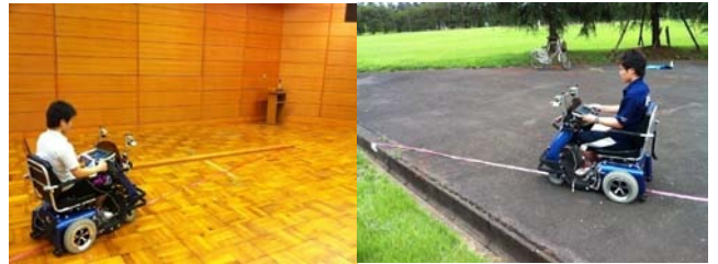
Fig. 3 Approach test (curb, gutter)
