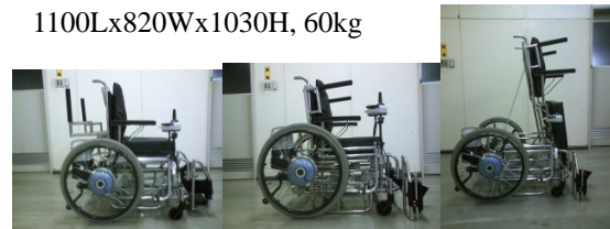
(a)Driving mode (b)Gait orthosis attaching mode (c)Standing position walk mode
