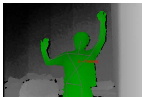
Fig. 2 Skelton extracted by Kinect sensor.
