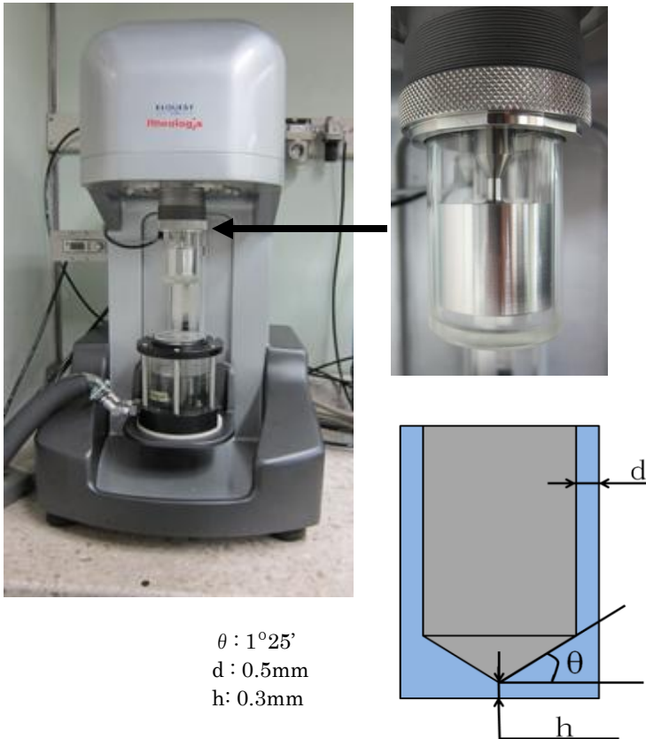
Fig.1 Observation and Cross-section of the shearing portion of a new rheometer
