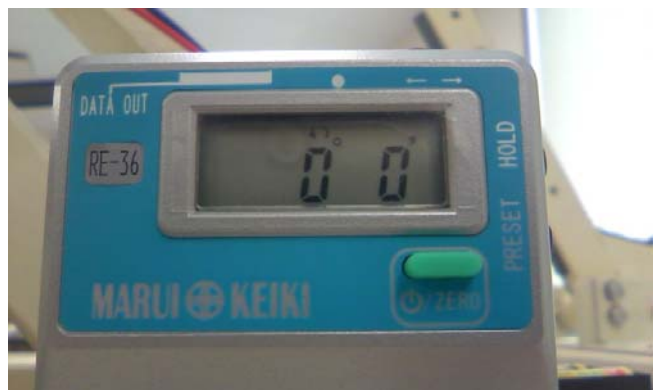
Fig.4 Shows the photograph of the digital goniometer. The sensor part of the goniometer is fixed on the top of the right arm of the exercise machine to synchronize the rotation as the arm.
