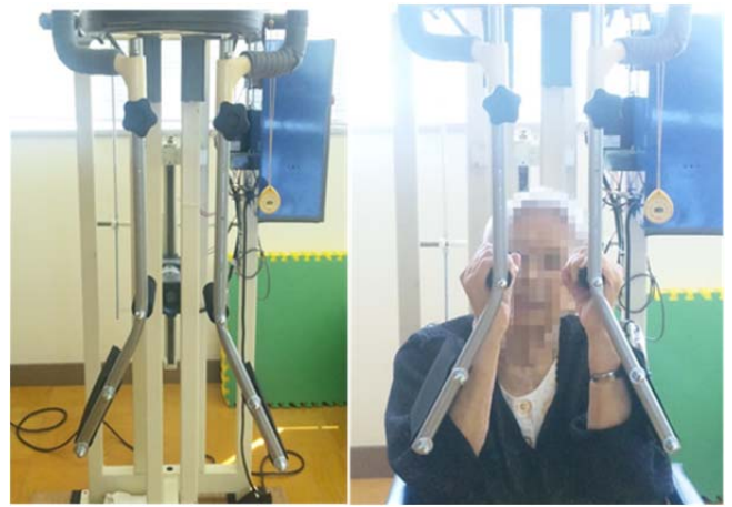
Fig.3 Shown is the photograph of the arm. The arm is 15 degrees bent from the position of handle and soft pad is patched at the elbows to avoid unexpected expansion during exercise.
