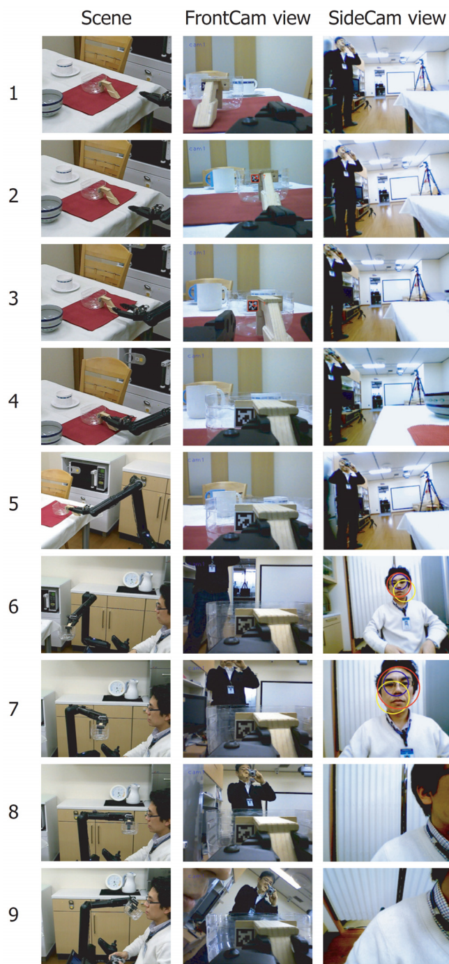
Fig.8 Two camera views in autonomous cup grasping and bringing
