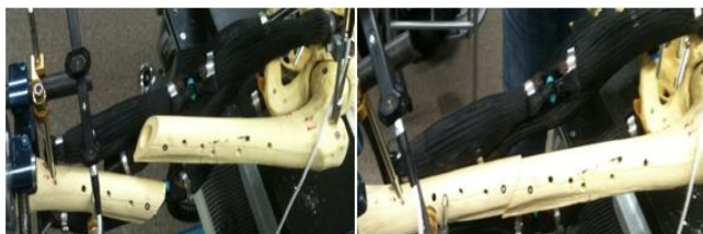
Fig. 2 Initial (left) and end (right) position of the distal and proximal fractured bone pieces
