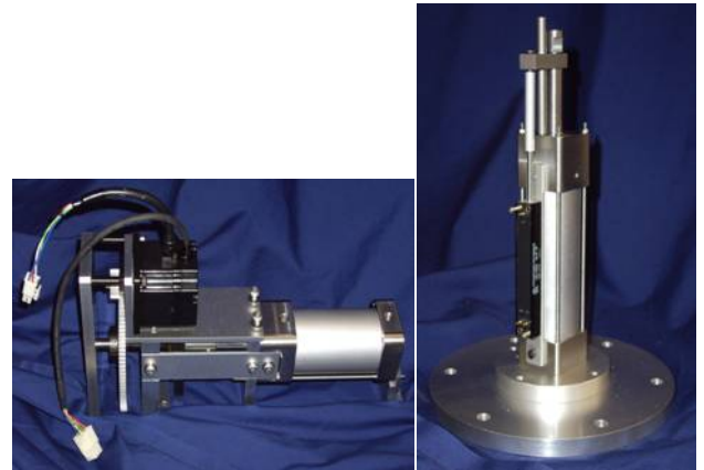
(a) Master Cylinder (b) Slave Cylinder Fig.2 HBSS for Vibration Isolation System
